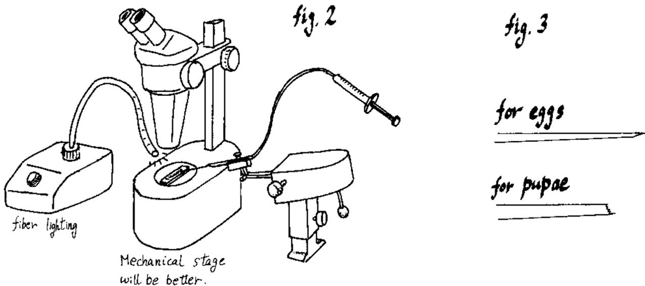
3. Break the tip of the needle with fine forceps under the microscope. Since the needle must penetrate thick pupal cases, the tip should be rather thick and robust (Fig. 3). Grinding the tip is not needed.
